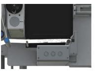
After printing, the label is cut to the desired length. The modified guillotine technique delivers a service life of several million cuts and simple blade changing.
