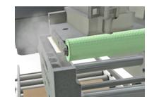
Not until the label is dispensed is the adhesive activated by precise jets of atomised water. The strength of the immediate, uniform and tenacious adhesion enables the label to hold fast for its lifetime.
